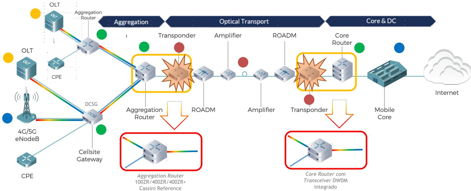
DCSG: Disaggregated Cell Site Gateway
